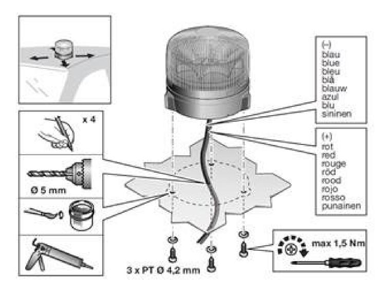
During installation of the fixed body variant make sure that the cables passage to the Interior is sealed. This can be done, for example, with a suitable rubber grommet or body sealant.
