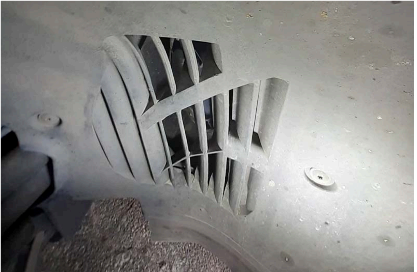
Figure 2: The fans can be accessed from the wheel well if the wheel well trim is removed first.
