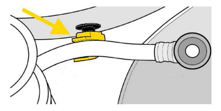
Inadequate fastening of the brake booster vacuum line caused by a faulty retaining clip.
