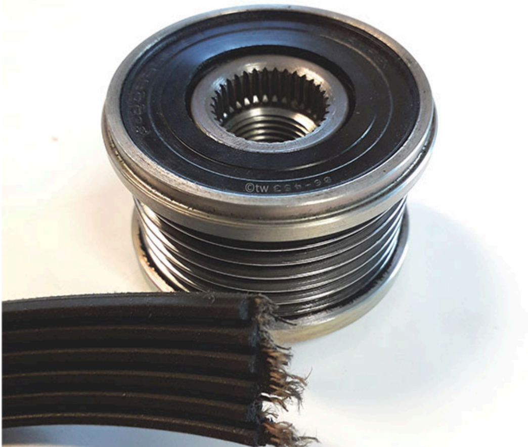
Defective overrunning alternator pulley with torn V-ribbed belt
