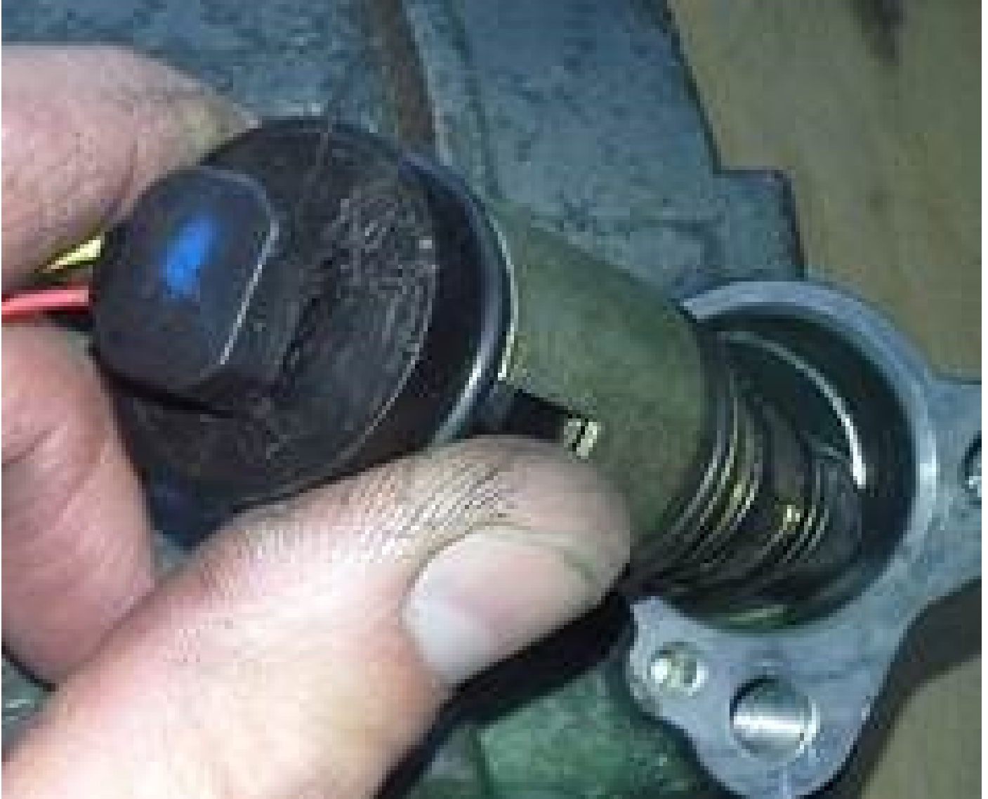
The figure shows an example of an electronically actuated pressure control valve
