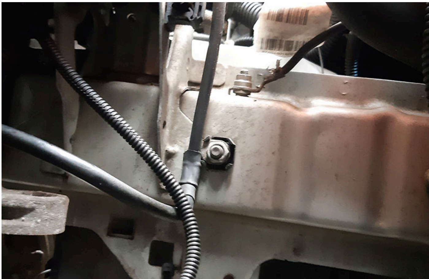
Fiat Grande Punto - engine does not start: Check ground connection
