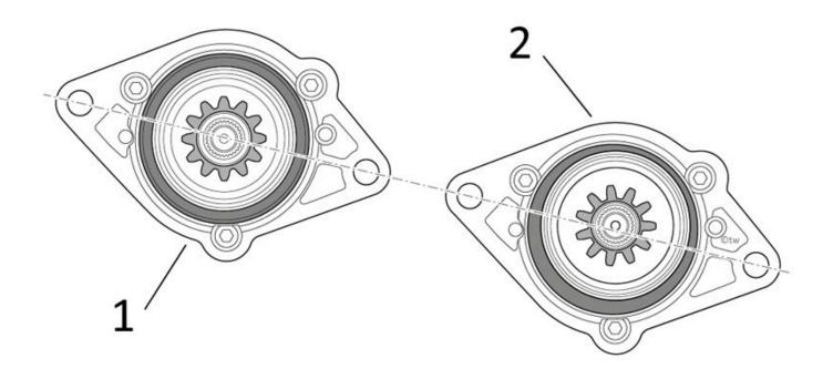
Starter with central (1) and offset (2) pinion position
