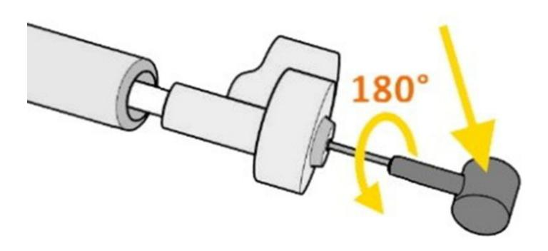
Turn the inner cable on the barrel nipple 180° anti-clockwise
