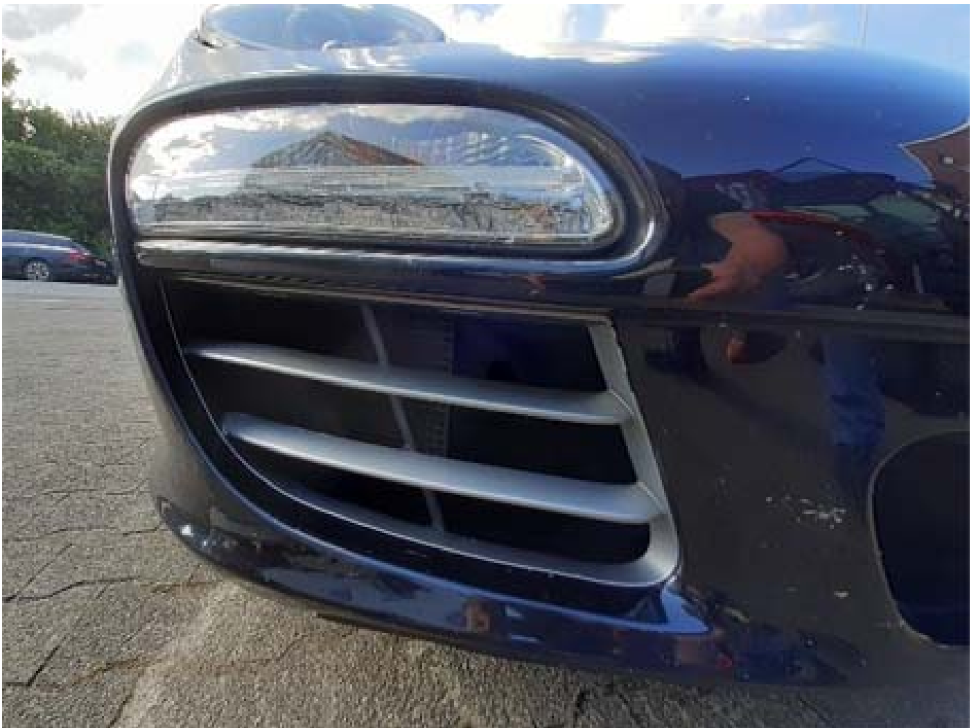
Figure 1: The radiators are located on the left and right behind the air guide grille in the bumper.
