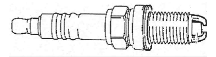
• Thermal overload can be caused by not properly tightened spark plugs. Consequential damages, such as defects in the centre and/or earth electrode and/or the insulator base by loosening or vibration of the spark plugs.
