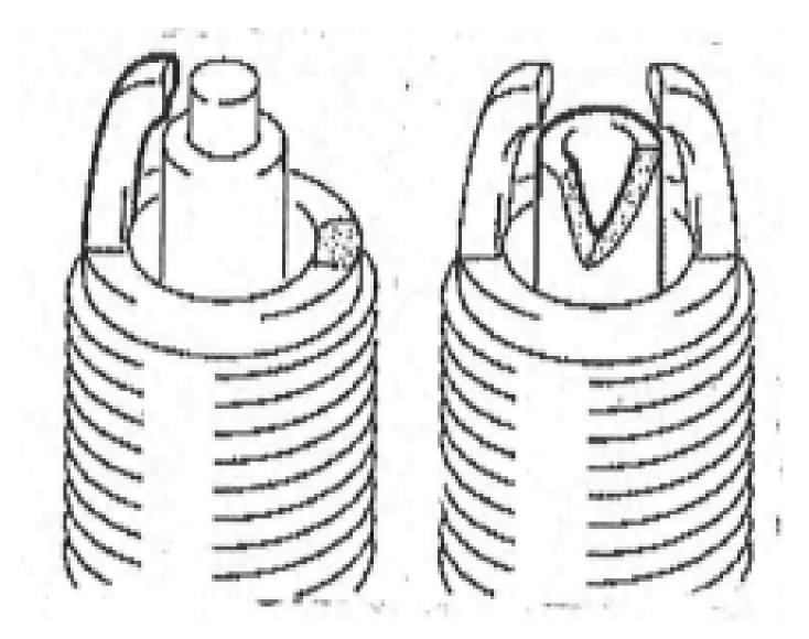
Fault patterns and possible causes (tightening torque too high):
