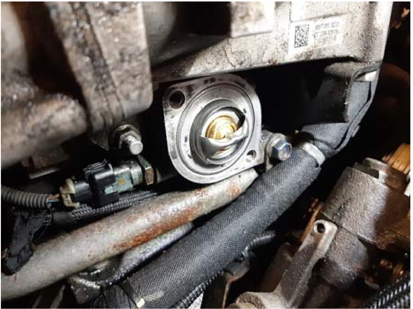
Figure 2: Thermostat visible and ready to be replaced
