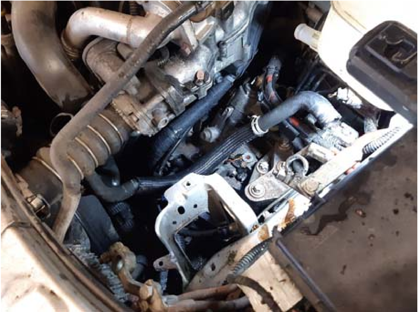
Figure 1: Removing the battery and battery bracket
