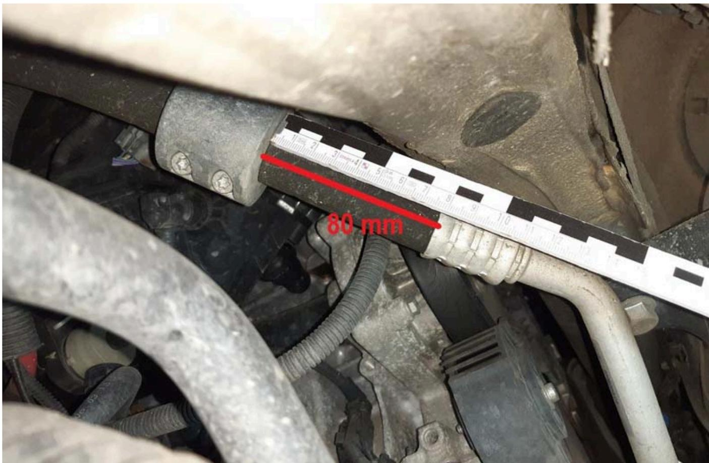
Figure 2: Install the vibration damper approx. 80 mm from the hose connection's crimping
