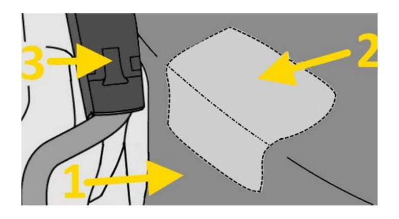
Picture 1: Permanent contact between the plug connection of the side airbag and the seat backrest upholstery
