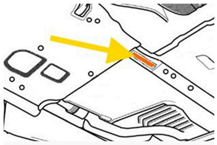
Thoroughly clean the area marked in the picture and fit the foam pad OE No. 16111181918 according to the vehicle manufacturer's instructions.
