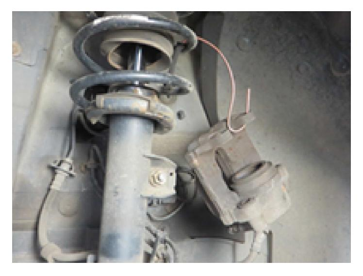
Loosen and unscrew the two fastening screws of the brake calliper carrier.
