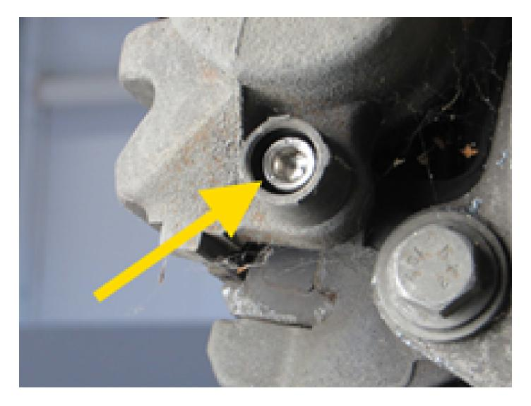
Remove the brake calliper from the brake calliper carrier.
