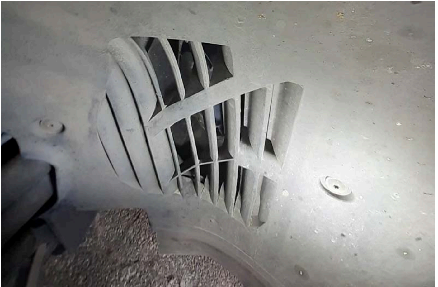
Figure 2: The fans can be accessed from the wheel well if the wheel well trim is removed first.
