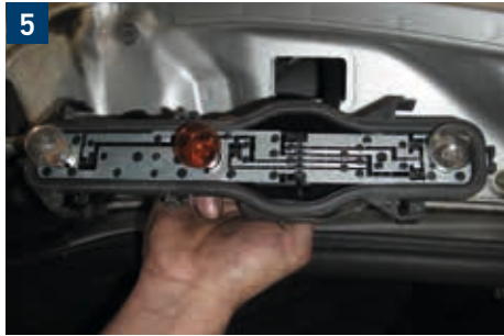
4 Position light, stop light, direction indicator light, fog light and reverse light (Rear lamp)
