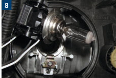
8 → For the low beam, pull the lamp backwards out of the reflector together with the plug.
