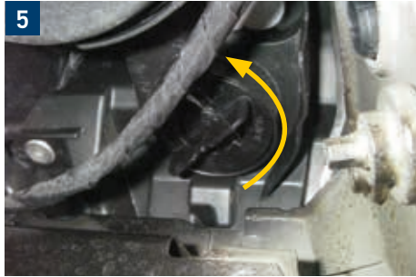
5 High beam and parking light (passenger side)
