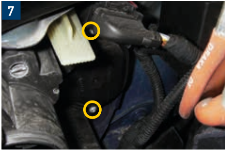
7 High beam and static dynamic cornering light (driver side)
