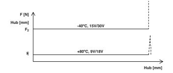
With a controller time of t1, the actuator has an actuating force of F1 < F < F2. The constant actuating force on the tappet over the rated stroke depends on the operating voltage and ambient temperature. If the actuator has no load to move over the stroke, the actuator power is converted into a higher actuator speed, resulting in the dynamic impact pulse becoming a multiple of the constant actuating force.
