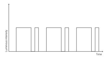
Intensive perception thanks to double-flash signal, 360° warning effect, rapid increase in light values, signal is clearly visible.
