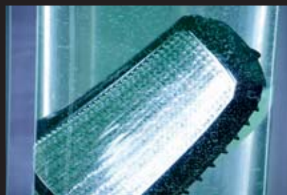
Immersion and leak test
